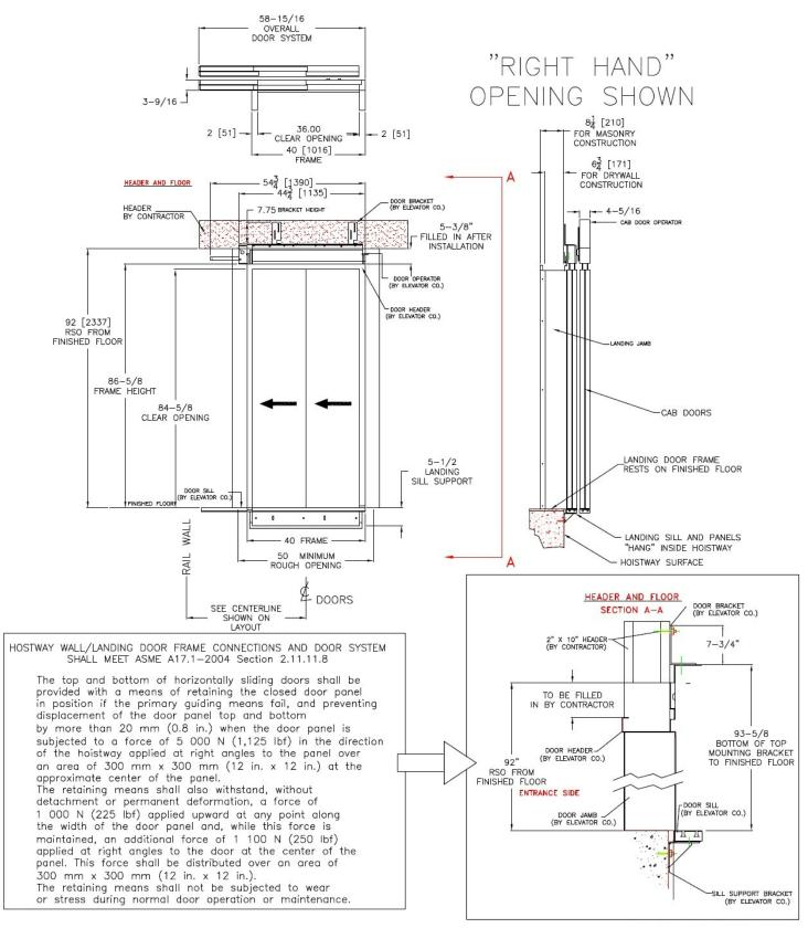
HOISTWAY WALLS AT ENTRANCES ARE TO BE BUILT AFTER DOOR SILLS AND FRAMES ARE SET IN PLACE. IF THIS IS NOT FEASIBLE, LEAVE A 50" X 92" ROUGH OPENING AT THE CENTERLINE AS SHOWN ON LAYOUT.
