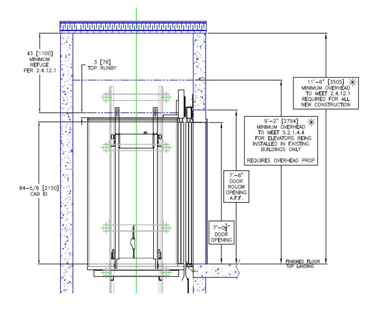
NOTE – ONTARIO ELEVATING AND AMUSEMENT DEVICES SAFETY DIVISION <u>CODE ADOPTION DOCUMENT #250/1 (1NOV2011)</u> PERMITS ALL LULA ELEVATORS IN ONTARIO TO MEET 5.2.1.4.4 BY UTILIZING OVERHEAD PROPS TO PROVIDE REFUGE, REGARDLESS IF NEW OR EXISTING BUILDING. AT LEAST 120" IS PREFERRED – 110" IS ABSOLUTE MINIMUM. THERE IS AN EXTRA CHARGE FOR ELEVATORS REQUIRING AN OVERHEAD PROP.
